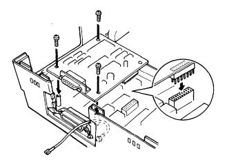
3. Attach the plug end of the FG wire onto the FG pin located on top of the interface board.
